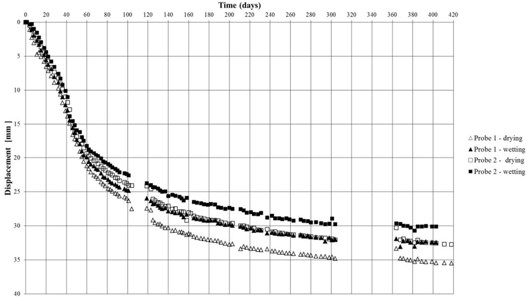
Figure 4. Change in height of test sample 2 (probes 1 and 2) after drying stage and wetting stage
