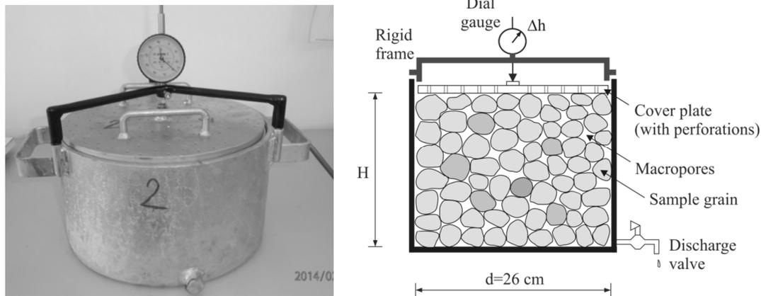
Figure 1. Testing cylinder
