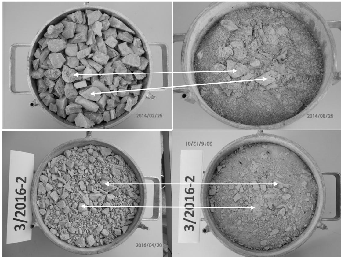
Figure 2. A view of the upper surface of test samples: 1- above, 3- below; before the test (left) and after the test (right)
