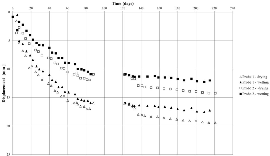
Figure 5. Change in height of test sample 3 (probes 1 and 2) after drying stage and wetting stage
