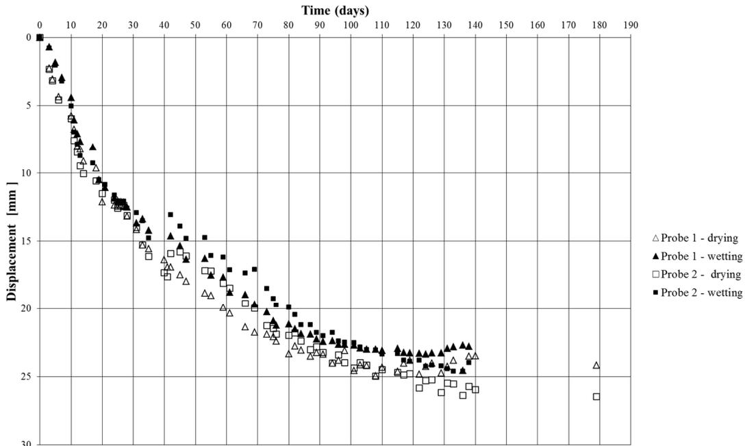
Figure 3. Change in height of test sample 1 (probes 1 and 2) after drying stage and wetting stage
