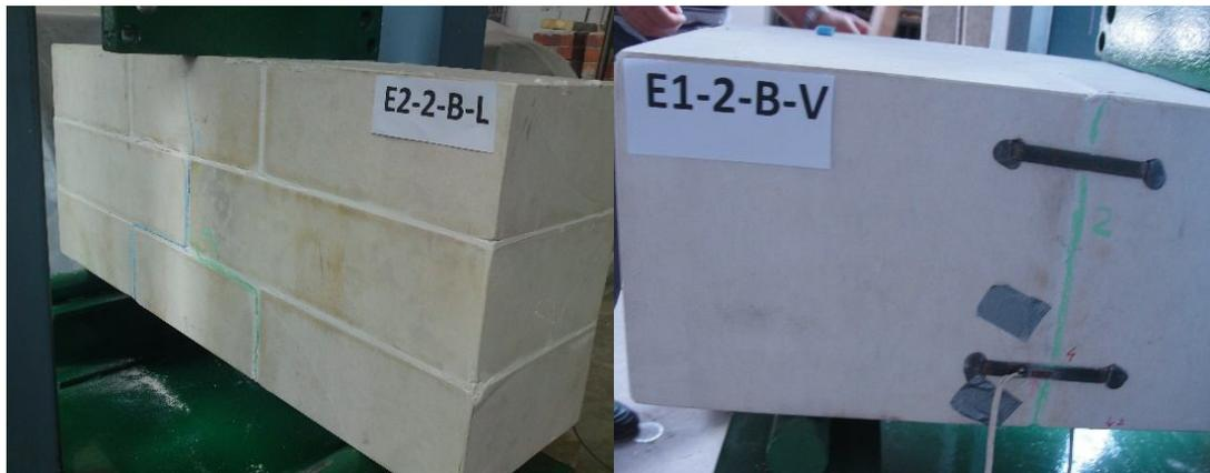
Figure 9. Occurrence of the first cracks in mortar joints
